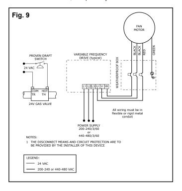
RSIB 350-500 can operate at either 3x208-230 VAC or 3x440-480 VAC (default). The motor wiring terminals shown in Fig. 10 shows default jumper positions for 3x440-480VAC operation.
